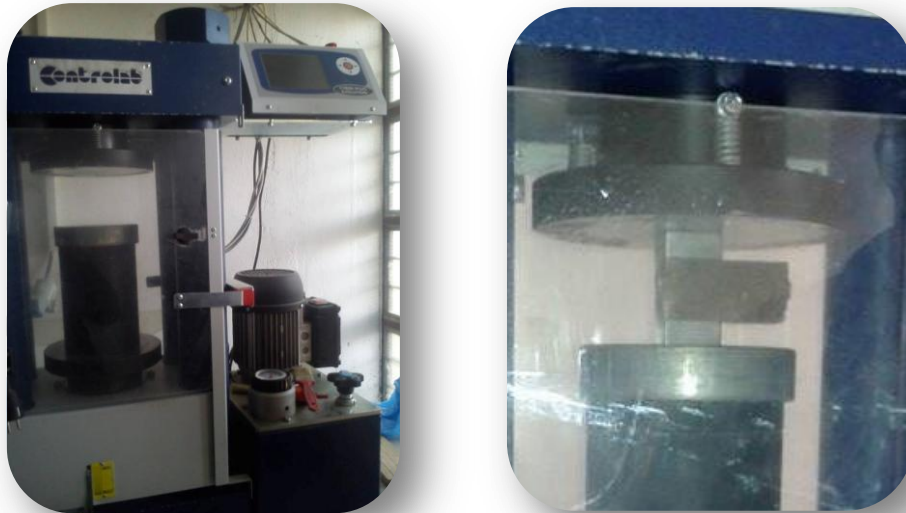
Figure III.12 : Appareille de compression (LNHC).
