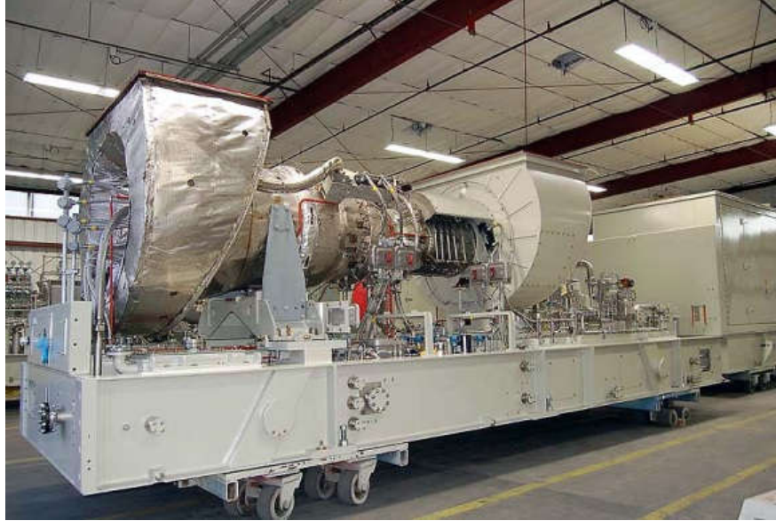
Figure III.37 : Turbine Solar TITAN 130
