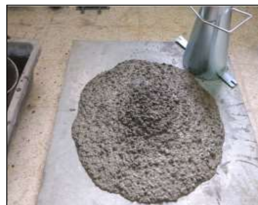
Figure 7. Slump flow test for fresh HPFRFC mixes.
