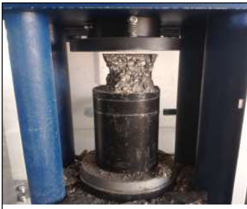
Figure 8. Compressive strength test for hardened HPFRFC mixes.
