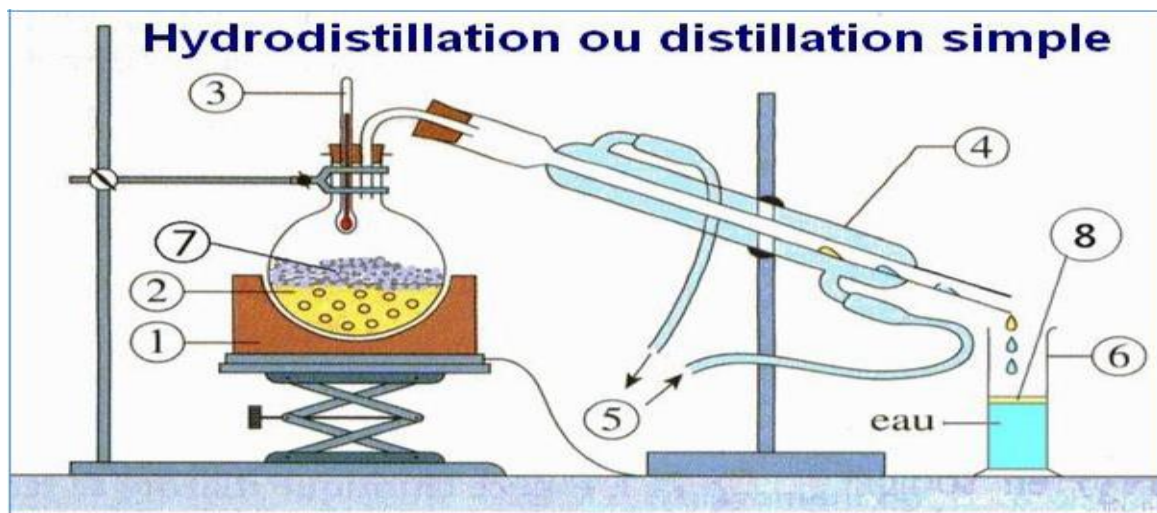
Figure 17 : L'hydro distillation (Jouault, 2012)
