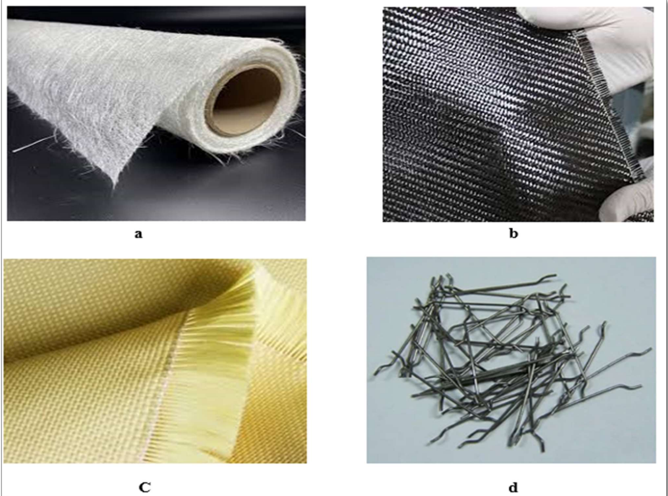
Fig 2. 8: type of fibers (a: glass , b: carbon , c: Aramid , d: steel )
