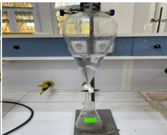
Figure17: Extractions liquide – liquide
