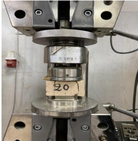
Figure II.16: Experimental Scene: Mechanical behavior of adobe bricks under compressive.
