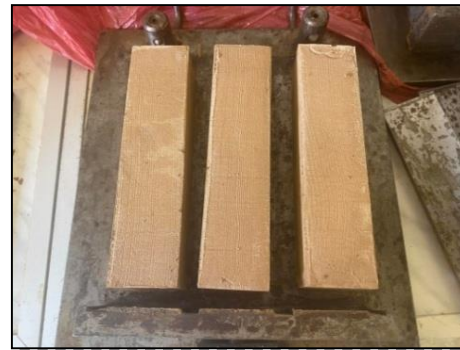
Unmolding of prismatic bricks
