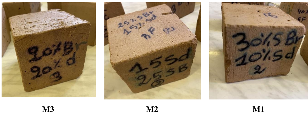
Figure IV.9: The mass loss of M3, M2, and M1 in cycle number 12.
