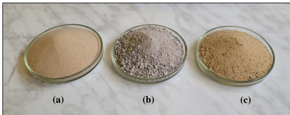
Figure II.8: Sands used in this study: (a) Dune sand, (b) Crushed sand, (c) River sand.
