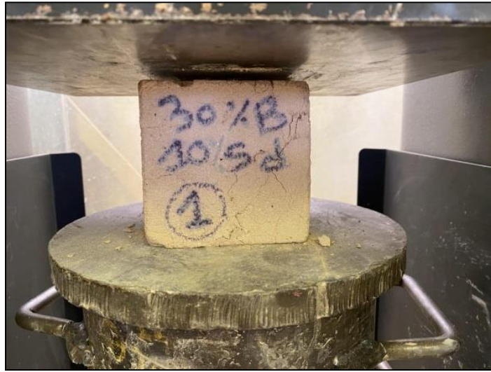
Figure II.11: Compressive strength test.
