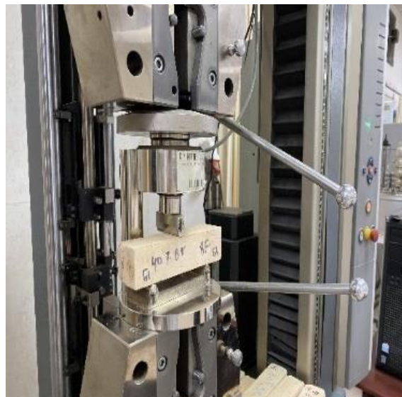
Figure II.16: Experimental Scene: Mechanical behavior of adobe bricks under compressive.
