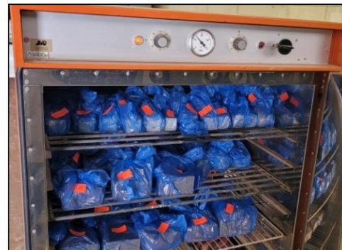
Curing in the oven
