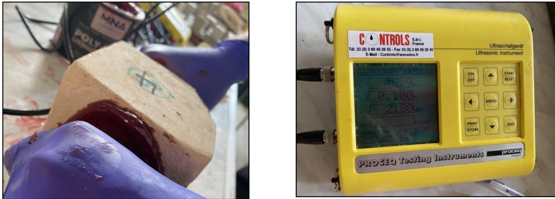
Figure II.15: Sound wave propagation speed test.
