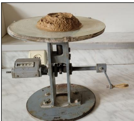
Testing on the flow table
