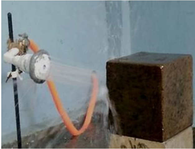
Figure I.23: Spray erosion test [47].
