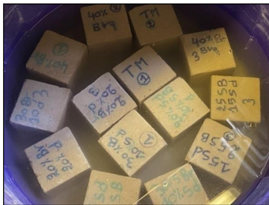
Figure II.13: Total water absorption test.
