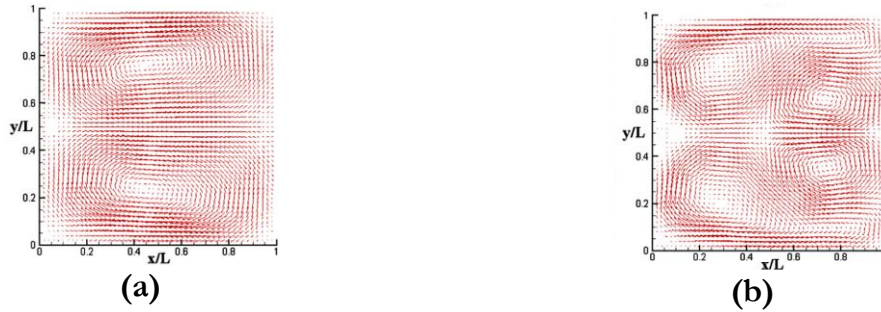
Figure 1.10: The effect of power-law index, n , on the velocity vectors of curved channel: (a) n = 0.8 , (b) n = 1.2 [27].
