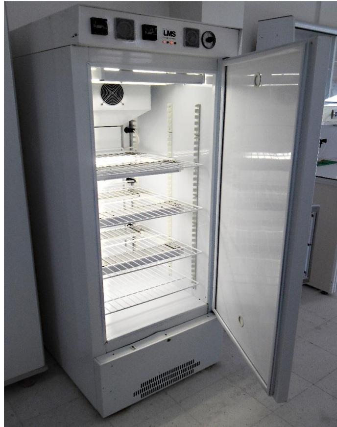
**Figure 1.** Incubateur (LMS Cooled Incubator)
