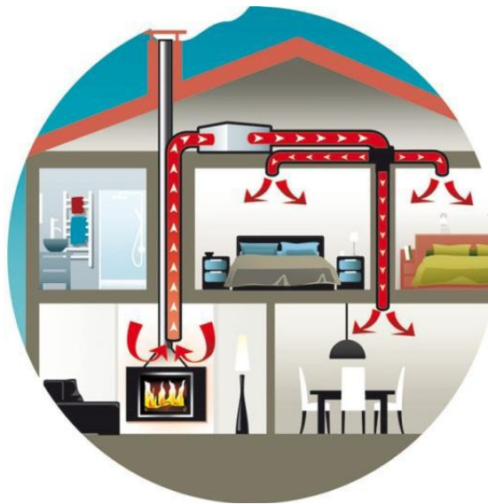
Figure I.1. Example of thermal recovery
