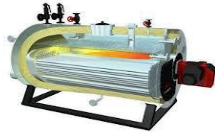
Figure III.8. Smoked tube boiler
