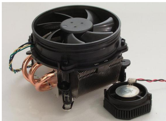
Figure I.4. Computer processor heat sink with copper heat pipe.
