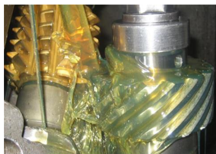
Fig. I. 1.13: Hobbing helical gear
