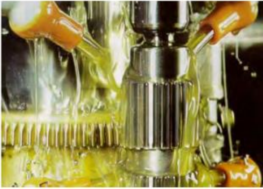
Fig. I. 1.15: Gear cutting: pinion
