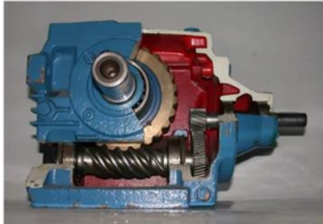
Fig. V. 1. 6: Worm and wormgear reducer
