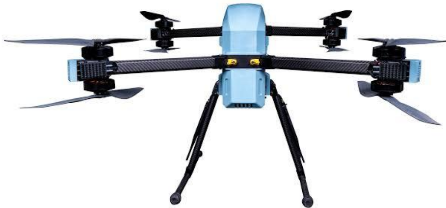
Figure I.3 Coaxial octorotor configuration
