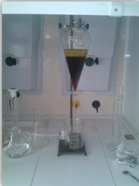
Figure 16 : Extraction liquide-liquide.
