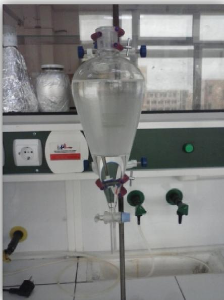
**Figure 11 :** Extraction liquide-liquide.
