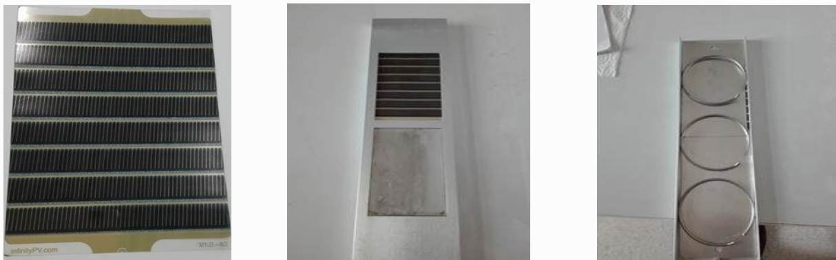
Figure III.1. (a) the organic solar cell before degradation, (b) the cells in support of QUV on face, (c) the support of QUV in front.
