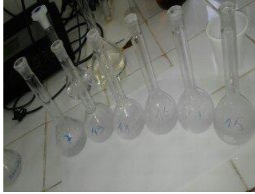
Figure 21: dosage de sulfate
