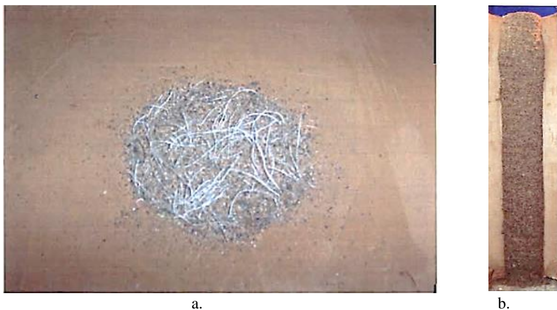
Figure 2.26: a- Top view of sand fiber mix pile after construction (upper view). b- Longitudinal section of pile after conducting the experiment “Problem of bulging” (side view)(Basu, 2009).
