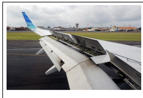
Figure I.27 : Spoiler system for a commercial aircraft [10].
