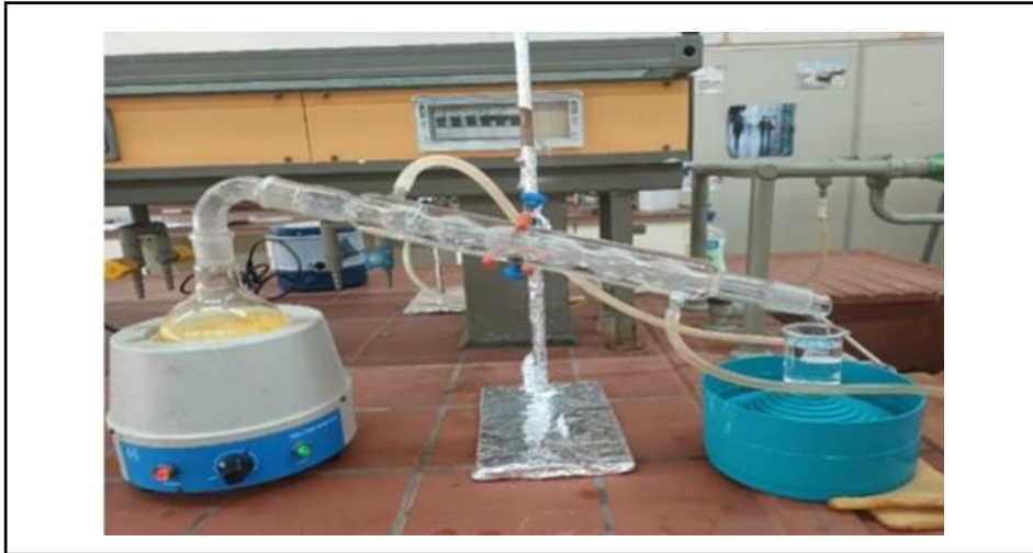
Figure 7: Montage de l'hydrodistillation. (Photo originale)
