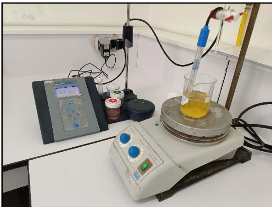
Figure 7. Titration of the sample using 0.1M NaOH (original image 2024).
